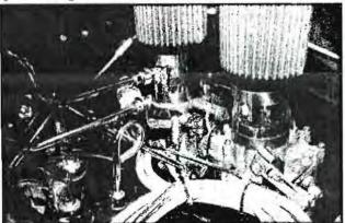
Here's a close-up of the throttle linkage and carbs on one side of the engine.
