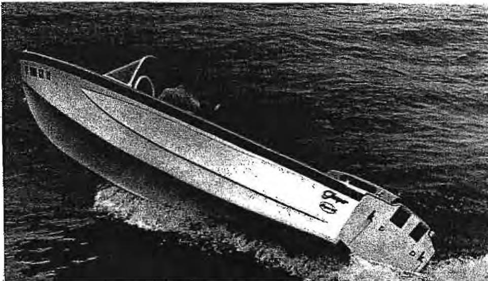
**ABOVE** - Fantastic bottom end torque will lift three adult skiers on single sticks in 35 feet from deep water. Boat loses only 8 mph at top end. **LEFT** - Punching throttle with rudder 'hard over' demonstrates the outboard-like maneuverability of the 16-foot Glaspar hull with the Corvaire pancake six.
