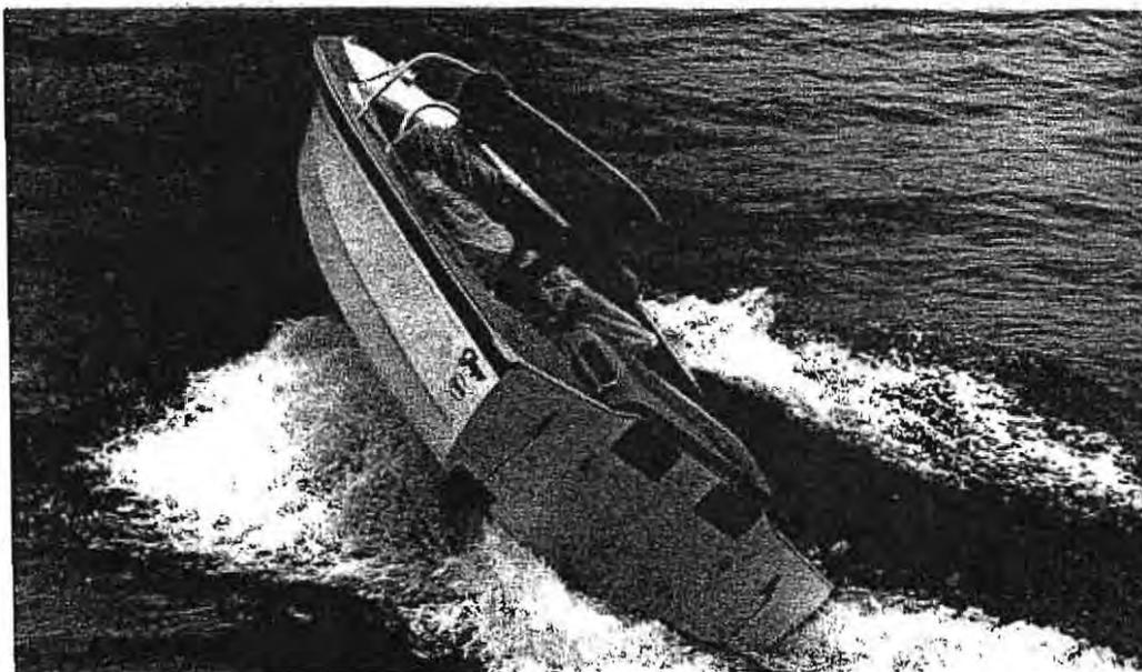
*This type of quick maneuver will sometimes bury the inboard rail, so be careful. Hull seems to pivot around a point amidship, as the power unit is driving both forward, and lifting the stern at the same time. Cooling air is drawn in through side openings in the engine hatch cover. Hot air is ducted through the transom along with exhaust; engine compartment is pressurized.*
