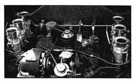
The SS engine is one classy looking unit. The fan housing and the alternator are done in a black wrinkle finish. This is nice looking but would be a pain to keep clean. The bare metal parts are all chromed.
