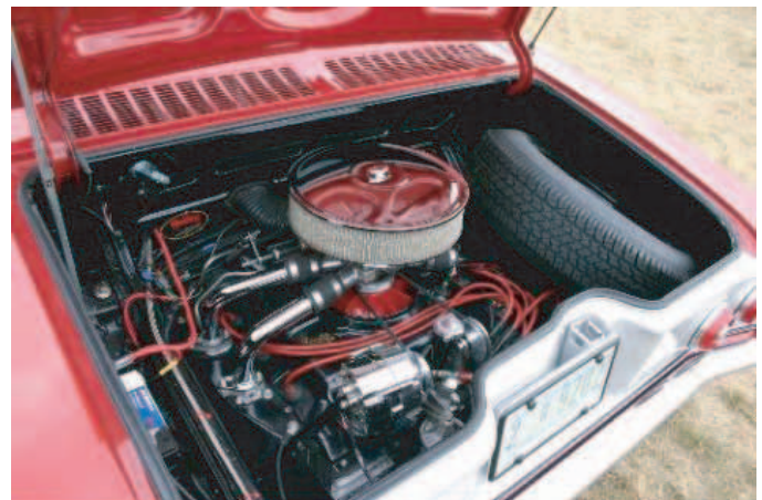
Above: One carb into four ports. Below: Four carbs into one air cleaner.
