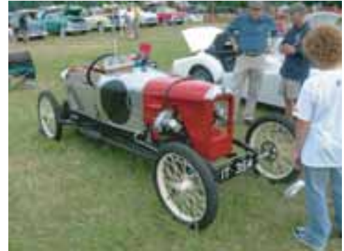
1920 GN Cyclecar V-twin, belt drive, made in London.
