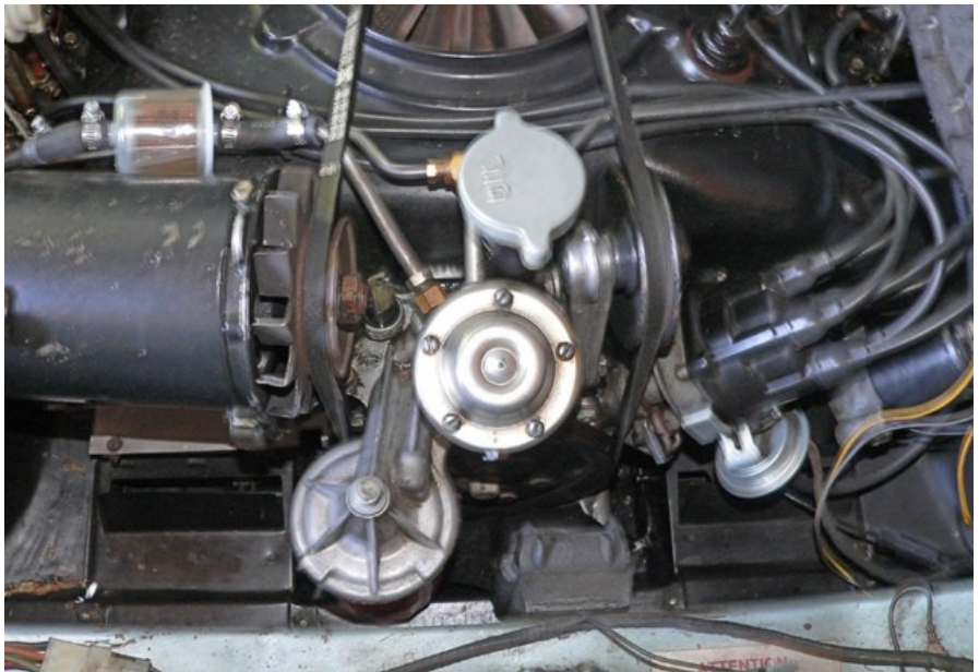
Photo # 1. This fuel pump mounted on a 1963 Corvair 102 hp engine is one of the "Bad" pumps that failed at 1,010 miles. You can tell by its extra shiny cover and the larger hold down screws. It is also made from heavy pot metal at nearly double the weight of an AC Delco fuel pump.
