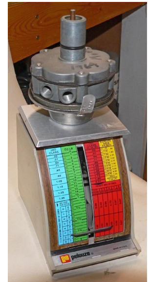
Photo # 3. This fuel pump is the replacement fuel pump that has the silicone diaphragm with no fabric reinforcement. At 26 ounces, it is nearly double the weight of the AC Delco fuel pump. It can be rebuilt with a new kit from Antique Auto Parts Cellar.
