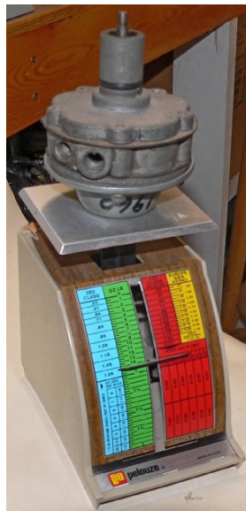
Photo # 2. This is a 1960 stock AC Delco fuel pump with the longer push rod and the light case, that weighs only 14 ounces, the preferred pump to re-build. The cover is only about half as shiny as the "bad" fuel pump.
