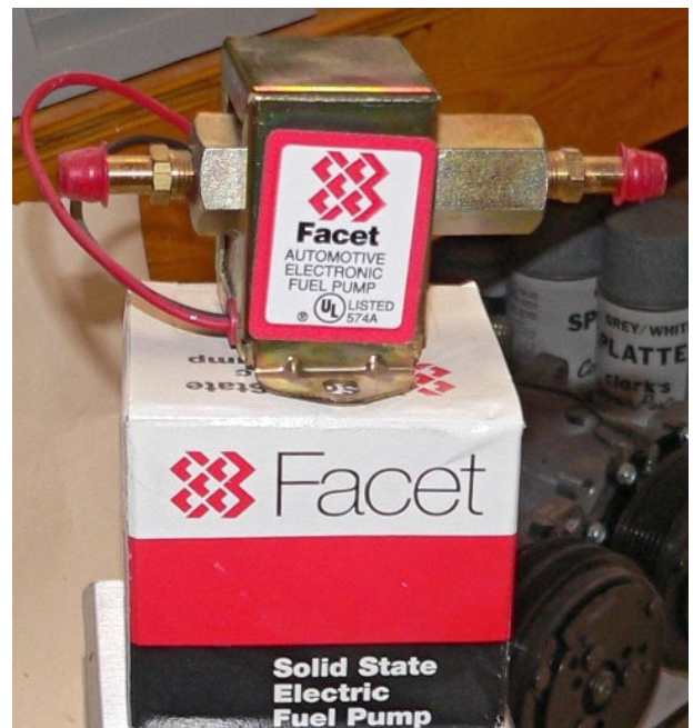
Photo # 4. This is a Facet brand electric "clicker" fuel pump that works well, other than the constant clicking sound it makes. The cost is about $45.00.
