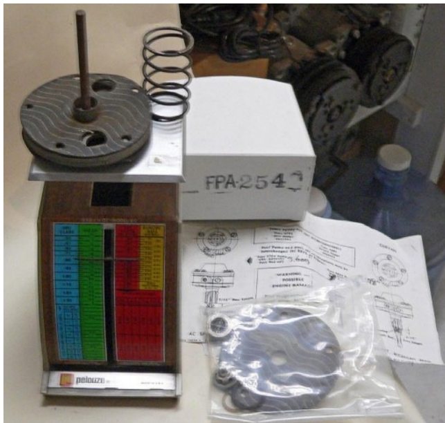
Photo # 6. Repair Kit. It is a good idea to mount a Fram brand plastic fuel filter just behind the alternator or generator to catch any dirt that could be in the fuel tank or fuel lines. These should be replaced about every 10,000 miles or less.
