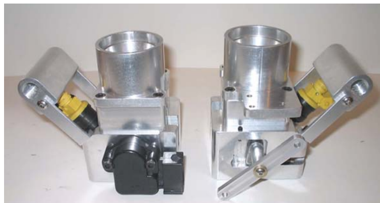
These throttle bodies use the original throttle linkage crossbar and air filter.
