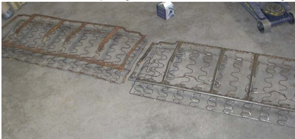
Original rust seat frame on the left and modified seat frame on the right.
