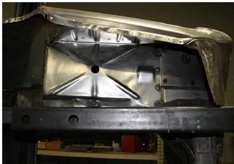
New sheet metal parts welded in place
