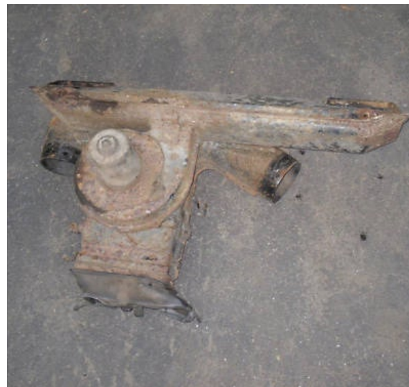
Early model heater box - to do a complete overhaul the engine has to be removed from the car to get the box out.
