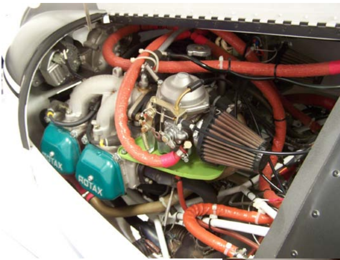
Above: The 100 horse-power Rotax opposed our cylinder engine isn't a Corvair but it pushed the P92 through the air at a steady 120 miles-per-hour.
