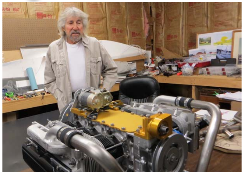
Ron Miles (above) explains a few of the modifications that had to be done to his '67 110-horsepower Corvair engine to make it flight worthy.
