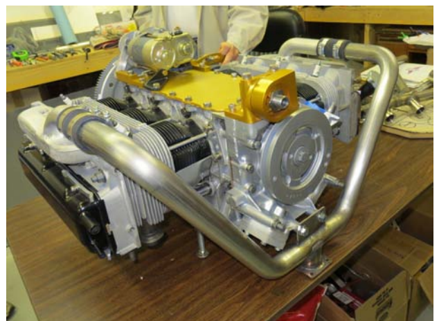
Ron Miles (above) explains a few of the modifications that had to be done to his '67 110-horsepower Corvair engine to make it flight worthy.
