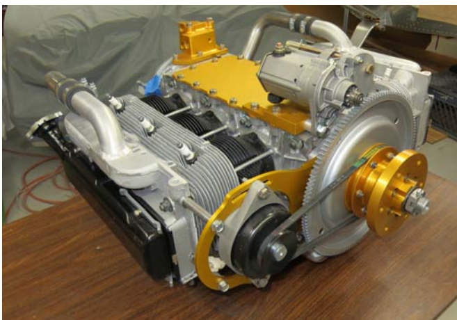
Below left: A view of the propeller-end of the engine showing the Subaru starter and special parts for mounting the prop and alternator. Below right: A view of the aft-end showing the special intake piping and oil filter adapter.
