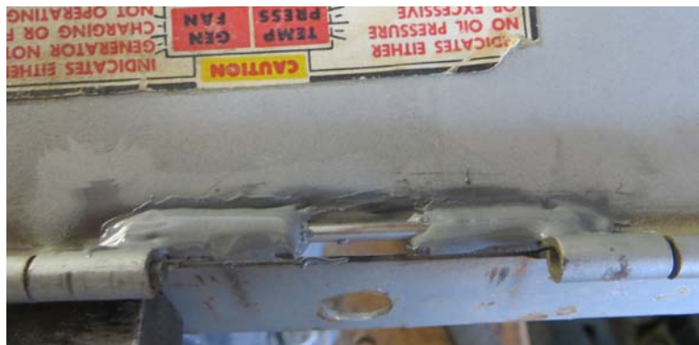
A 2" piece of welding rod which will serve as a support for the spring is held in place with J-B Weld.
