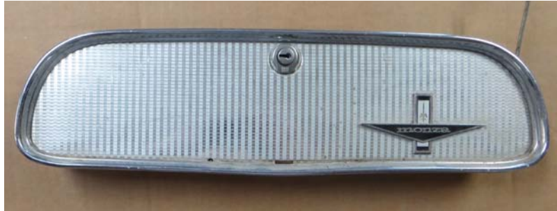
The early model glove box doors almost always end up with a bent trim piece.
