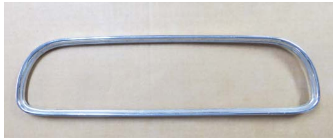
The trim piece can be straightened by carefully working it with a rubber mallet.
