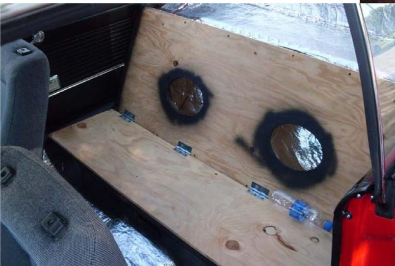
*Even though Mike has spent months on his project thus far, there is still a lot of work to be done. The wood grain (non-telescoping) steering wheel brings a nice look to the car's interior (above). The back seat has been removed and replaced with plywood which Mike has prepared for stereo speakers (left). Lots of sound proofing material has been applied throughout the interior of the car.*
