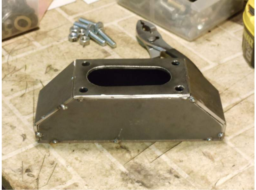
The photo above shows the basic plenum before final welding. Below, is the plenum with one of the Weber carburetors setting in place.
