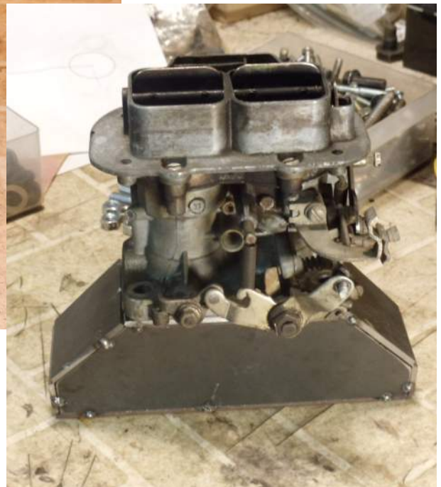
In the photo to the right, John has placed risers on the bottom side of the finish-welded plenum with carburetor base gaskets set in place to show what the final mounting layout will be.
