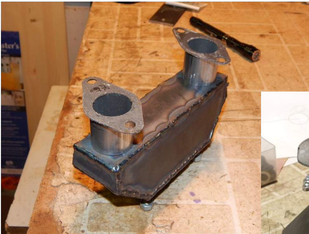
The photo above shows the basic plenum before final welding. Below, is the plenum with one of the Weber carburetors setting in place.
