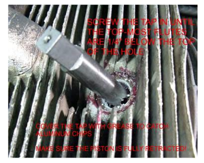
Once the top cutting surfaces are about 1/4" below the top of the hole, slide the seat cutter over the tap. The seat cutter has two sets of cutting teeth: one to cut a chamfer to mate with the flare on the top of the insert and one to cut a spark plug washer seat.
