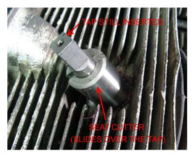
*Slide the seat cutter over the tap without removing the tape.*
