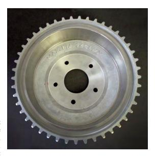
One last finishing touch, before installation, I mask and paint any steel drum weights (I use a light silver- gray Hammertone). Finding the aluminum brake drums is getting more difficult. I've found wrecking yard prices of up to \$125/ each for the GM front brake drums and \$30/each for the GM rear brake drums
