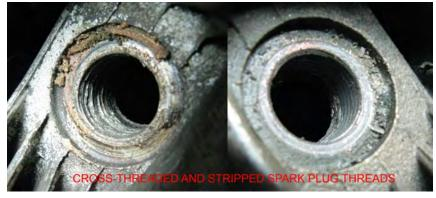
Use the step-tap to cut new, larger threads in the spark plug hole. The first set of threads on the step-tap match the existing spark plug threads, so this helps guide the tap. Apply grease to the end of the tap to catch the aluminum chips and be sure the piston is fully retracted to ensure you don't "tap" the piston.
