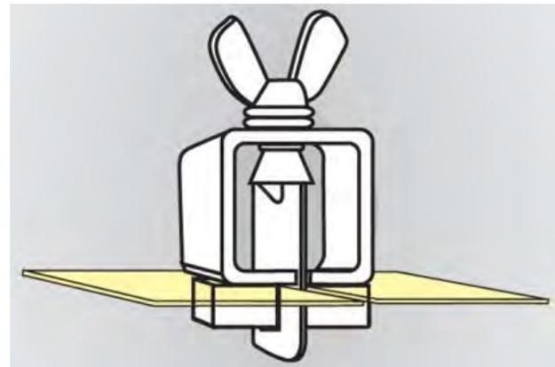
*In the case of replacing a rusted panel, the pieces can be clamped and welded with no need for any additional material to fill the gap since the blades on the clamps are only .040" thick.*
