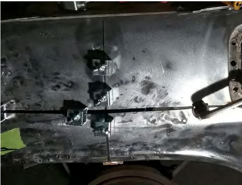
*Mike's project includes flaring the fenders to accommodate wider tires. He cut the sheet metal, spread it out to the desired width and used the clamps to hold things in place. In this case he will add filler strips since the gaps are too wide to fill with weld.*
