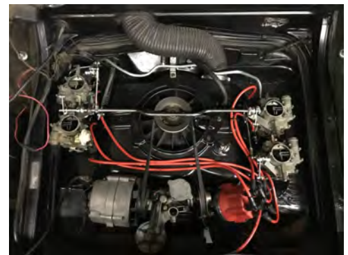
140 hp Corsa option: 4 single-barrel Rochester carburetors.
