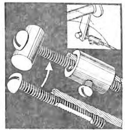
Broken clutch cables on four speed Corvairs can be repaired by sliding a sleeve over the cable, matching it with a No. 12-24 2" bolt held in the clutch-lever slot by a drilled \( \frac{1}{8}\)"-by-\( \frac{3}{4}\)" rod. The bolt threads grip the cable better than a pressed on tip.
