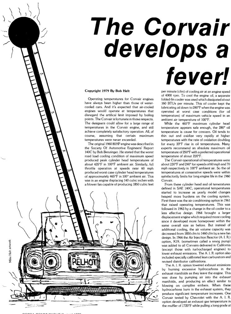
per minute (cfm) of cooling air at an engine speed of 4000 rpm. To cool the engine oil, a separate folded-fin cooler was used which dissipated about 160 BTUs per minute. This oil cooler kept the lubricating oil down to 280°F when the engine was operated at worst case conditions (for oil temperature) of maximum vehicle speed in an ambient air temperature of 100°F.
