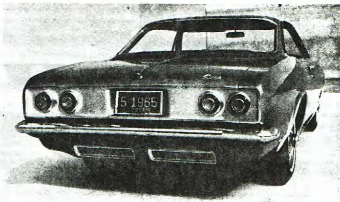
SCULPTURED TAIL bears family resemblance to bigger Chevrolets. Air inlets have been moved off deck lid into plenum chamber just below the rear window.
