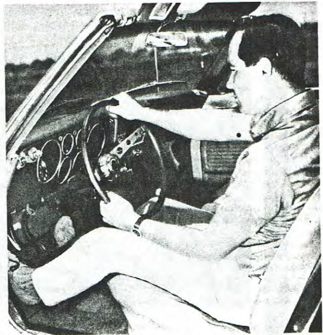
Optional adjustable steering wheel permits straight-arm driving position favored by many sports car buffs. Absence of front floor tunnel adds to interior spaciousness.
