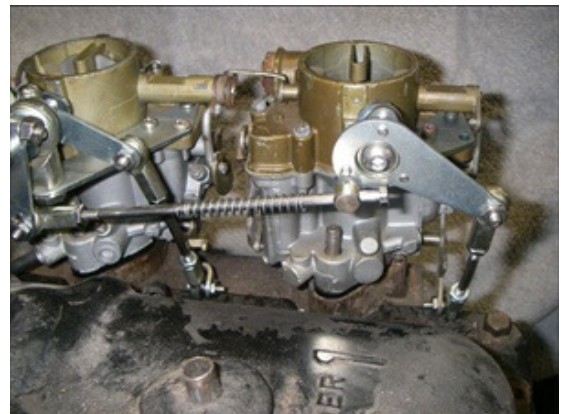
1966-69 140hp Right Side. Using Choke Lock-Outs.
