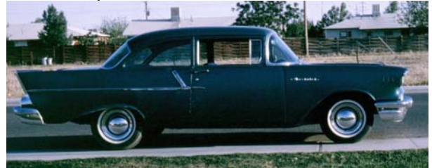
The 1957 Chevrolet 150 with the famous Blue Flame 235 and three in the tree.
