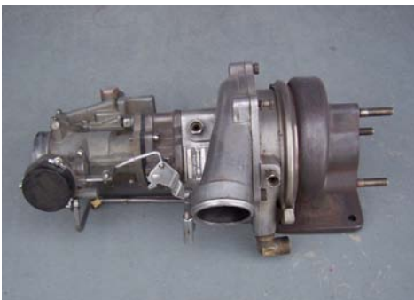
A late model turbocharger with carburetor ready for installation.
