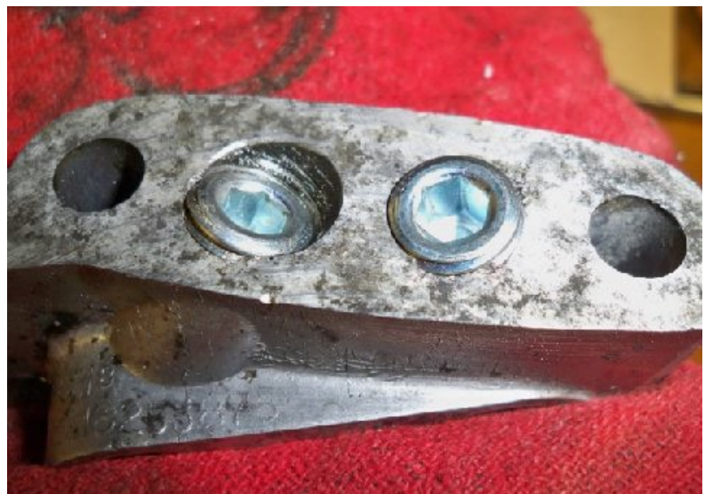
Drill out the two oil passage holes with a 7/16" drill and tap each hole with a 1/4" NPT tap.
