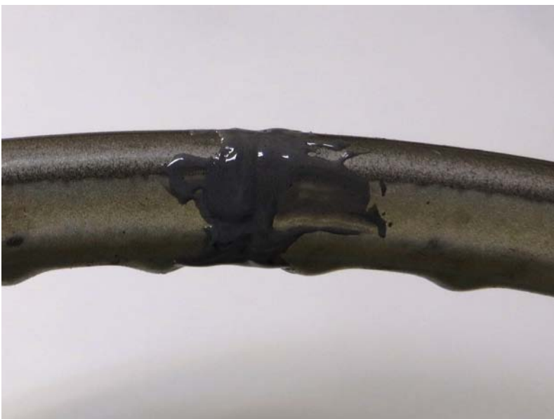
The grooves are filled with epoxy. J-B Weld works perfectly and is readily available. Allow the epoxy to cure at least 24 hours. Note: Use regular J-B Weld, not J-B Kwik. The fast setting stuff doesn't seem to ever get hard enough to sand very well.
