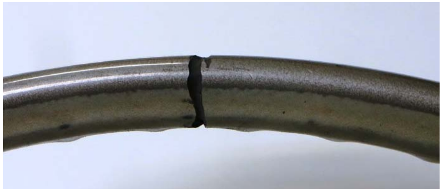
With a Dremel tool each crack is opened up. Putting a nice deep groove where the crack used to be allows space for the filler.
