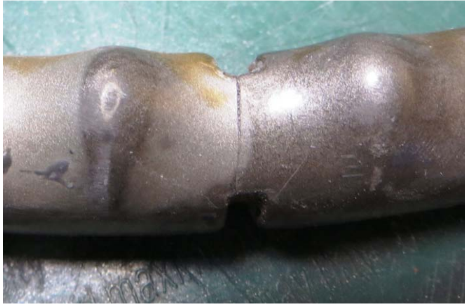
Here is just one example of one of the many cracks in this '62 Monza wagon wheel. There were about 25 cracks in all.
