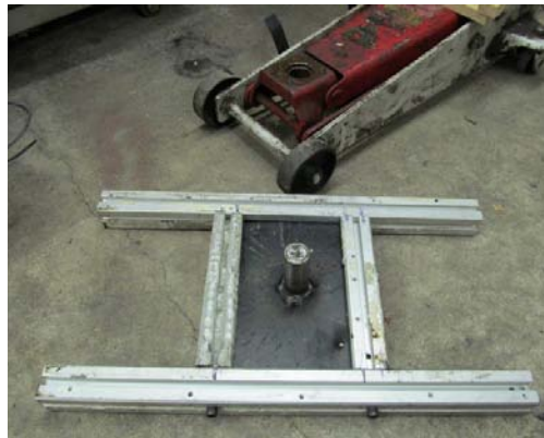
Left: A bottom view of the cradle showing the round steel bar welded in the center of the plate. The diameter of the bar needs to be able to fit into the hole in the floor jack.
