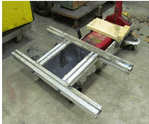
Left: The finished cradle on the floor jack. Below: The cradle in place ready to support the Corvair drive train.
