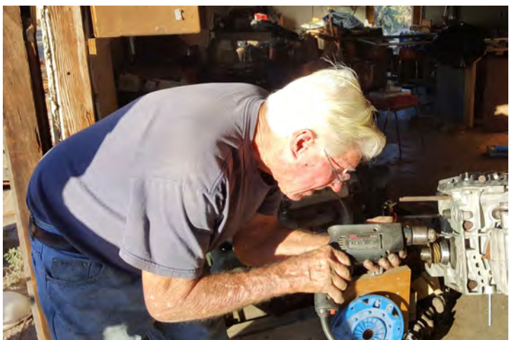
Bill Maynard teaches FJ Trejo the finer points of removing a broken bolt.
