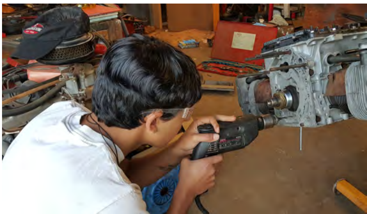
Bill Maynard teaches FJ Trejo the finer points of removing a broken bolt.
