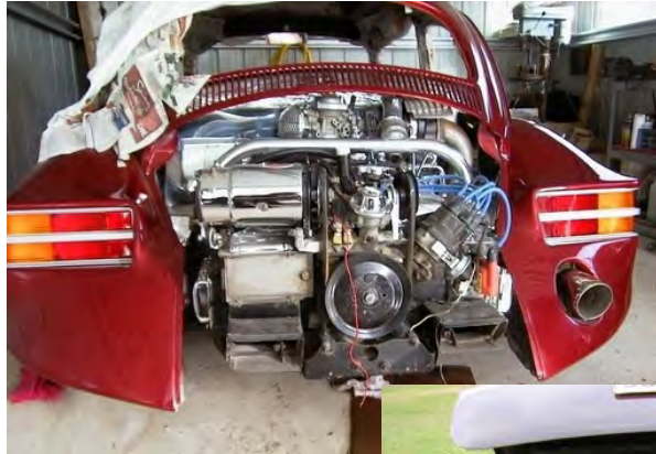
A unique example of a Corvair engine in a highly customized VW Beetle.
