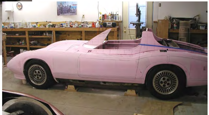
The chassis was shortened from a 108-inch to a 93-inch wheelbase (above). The foam body plug forming began and the car started to take the shape. The front and rear clips would be removable (right). The roll bar will be a separate piece.
