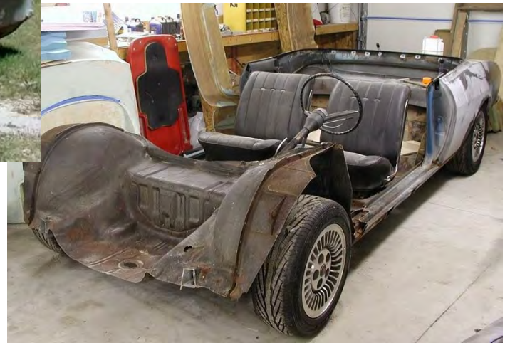
The project started life with this '65 convertible that had survived a barn fire that Mel got for free (left). Body panels were cut away but would be structurally reinforced with tubing (below).
