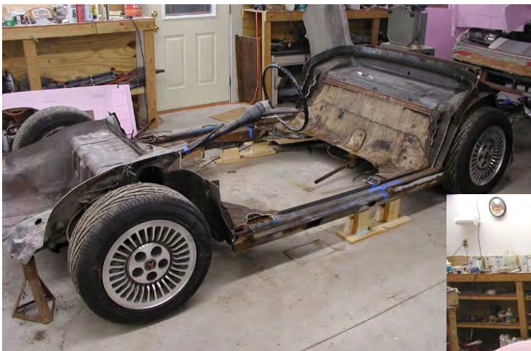
The chassis was shortened from a 108-inch to a 93-inch wheelbase (above). The foam body plug forming began and the car started to take the shape. The front and rear clips would be removable (right). The roll bar will be a separate piece.
