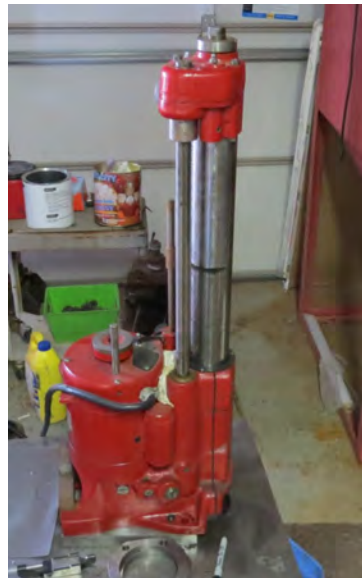
The equipment shown below is used for boring Corvair cylinders. The tag on the bottom indicated that it was shipped to Pearl Harbor in 1943
