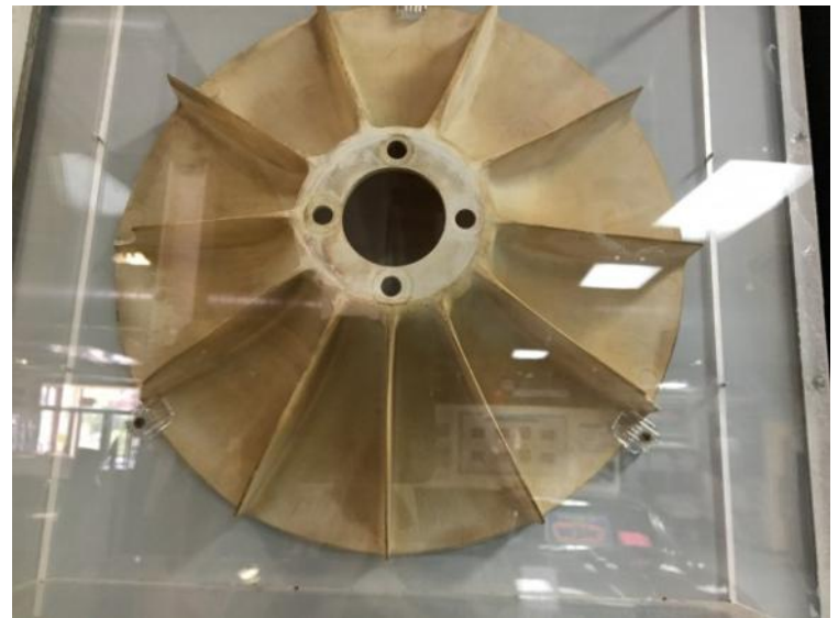
Even before production began, Chevrolet engineers were investigating ways to improve or replace the steel cooling fan. The old steel fans used up to 10% of the engine's horsepower at 80 mph. The fan shown here was scheduled to go into production in April 1962 for use on the Spyderys only. It was made of Delrin and was much lighter than the steel fans. In testing it was discovered that when Delrin was exposed to droplets of sulfuric acid from an over charged battery, formaldehyde was formed which wasn't too good for the occupants of the car when the heater was in use. Production was cancelled. In 1964 the plastic fan blueprints were used to manufacture the magnesium fan that we all know today.
