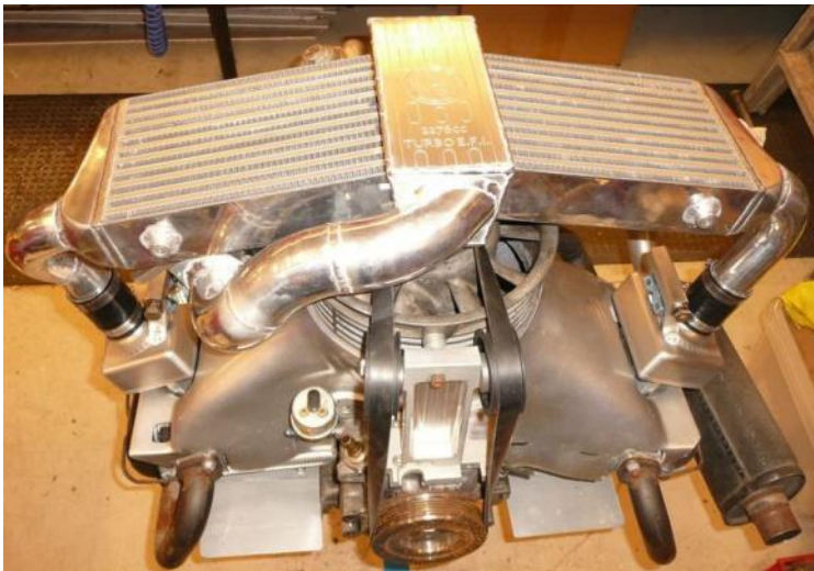
Not exactly a Corvair picture, but it shows how desperate Porsche people are to convert their systems over to the Corvair-type fan belt arrangement. Of course the Porsche folks can't use a standard V-belt when serpentine belts are so much more classy.
