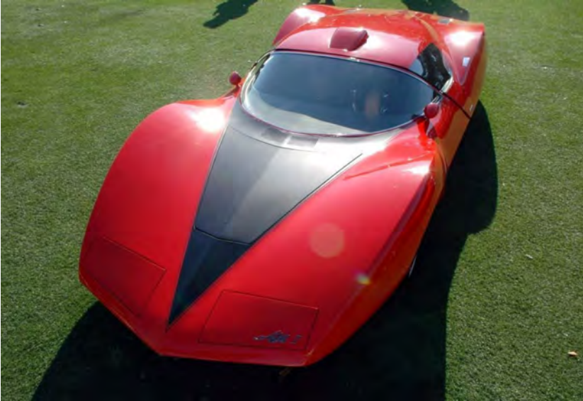
The Astro I was a concept car for the Corvette but the 35-inch tall vehicle has no room for the standard V8 engine so a highly modified Corvair power plant was used instead.
