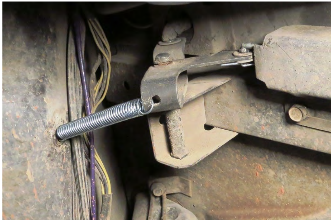
The new spring attaches in the stock original location. One end of the spring has to be trimmed off to about to slip into the sheet metal in the front. The other end has to be trimmed as well the able slip into the hole in the throttle lever.
