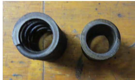
In both photos, the spring on the left is the stock Corvair valve spring. The one on the right is the "new and improved" spring. There was about and .001 inch end play in the smaller spring when installed. The engine must have had zero to very little compression.
