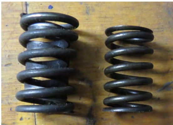
In both photos, the spring on the left is the stock Corvair valve spring. The one on the right is the "new and improved" spring. There was about and .001 inch end play in the smaller spring when installed. The engine must have had zero to very little compression.
