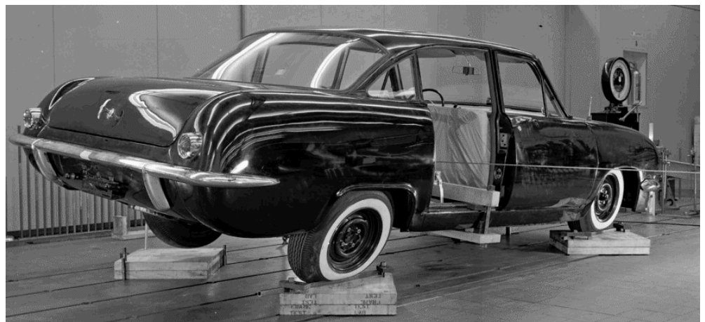
Testing torsional rigidity. Rear wheel "tuck under" is significant.
